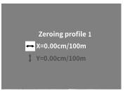
100 m. Confirm the setting by briefly pressing the menu knob **(5)**. Now make the settings for the Y axis in the same way. Switch between the setting for the X and Y axis by briefly pressing the menu button **(5)**.
