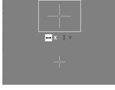
displayed enlarged in an additional window. Setting the X axis: Press the left arrow button (4) for minus and the right arrow button (4) for plus. Every time you press the button, you move one pixel further. To jump several pixels further, hold down the arrow button (4) longer. Confirm the setting by briefly pressing the menu button (5). Now make the settings for the Y axis in the same way. Switch between the setting for the X and Y axis by briefly pressing the menu button (5).
