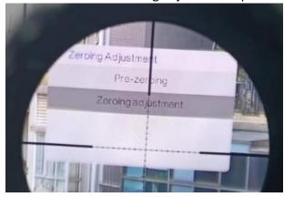
6. Adjust the X/Y axis to move the yellow cross to the aiming point before installing the FD/FT (aiming point in your Optical scope), then press the Menu key to return and save.
