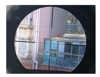
**Note:** After each installation of the FD/FT, you can double-click the menu key to confirm whether the red reticle(German version: Red dot) aligns with the optical reticle. The red reticle (Red dot) will automatically vanish after three seconds.
